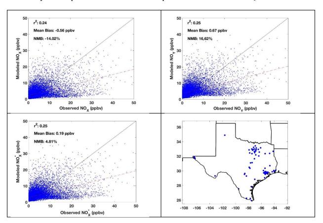
Preliminary first outputs from the 3-dimensional photochemical model CMAQ are shown below.
